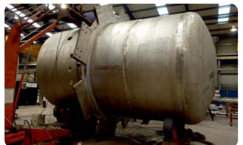
Lower Section of the Evaporator Vessel
