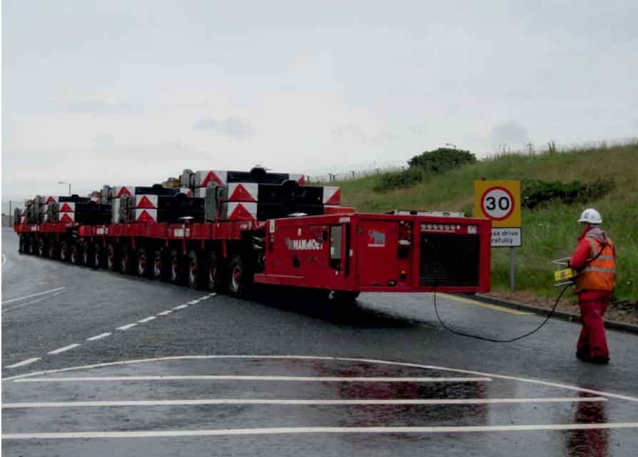
Self Propelled Modular Transporter
