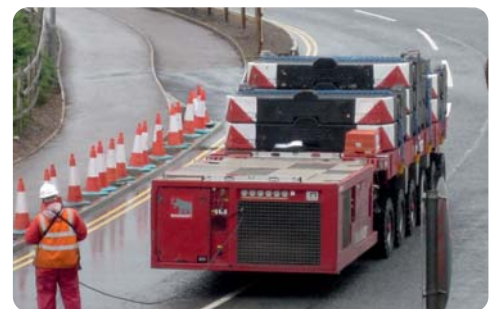
Self Propelled Modular Transporter
