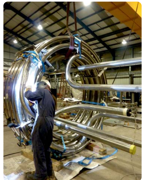
Welding of the Riser Section of the Evaporator Coil
